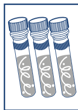
4. 3D beat-beating: same efficiency in each tube enables the liberation of cell components
